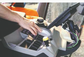
Control via operation panel
