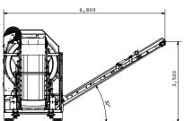
With a drum diameter of 2,200 mm and a hopper capacity of 6,5 m<sup>3</sup>, as well as conveyor belt discharge heights of 3,500 mm, the **Siebo 6000** is a benchmarking machine. It enables a high throughput performance at law operating costs in provative in its class is
